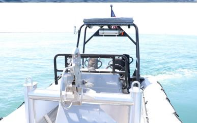
Lifting and self-righting frames allow for easier transferring of the vessel and security against unexpected emergencies at sea.
