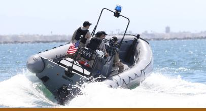
Coxswain backrest and stern storage box provide an open deck area to fit a maximum of 18 people on board with ample storage space.
